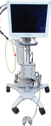
The CCD/LED camera attaches to the controller which has a focus knob for the camera and provides white balance, gain control and illumination settings.
