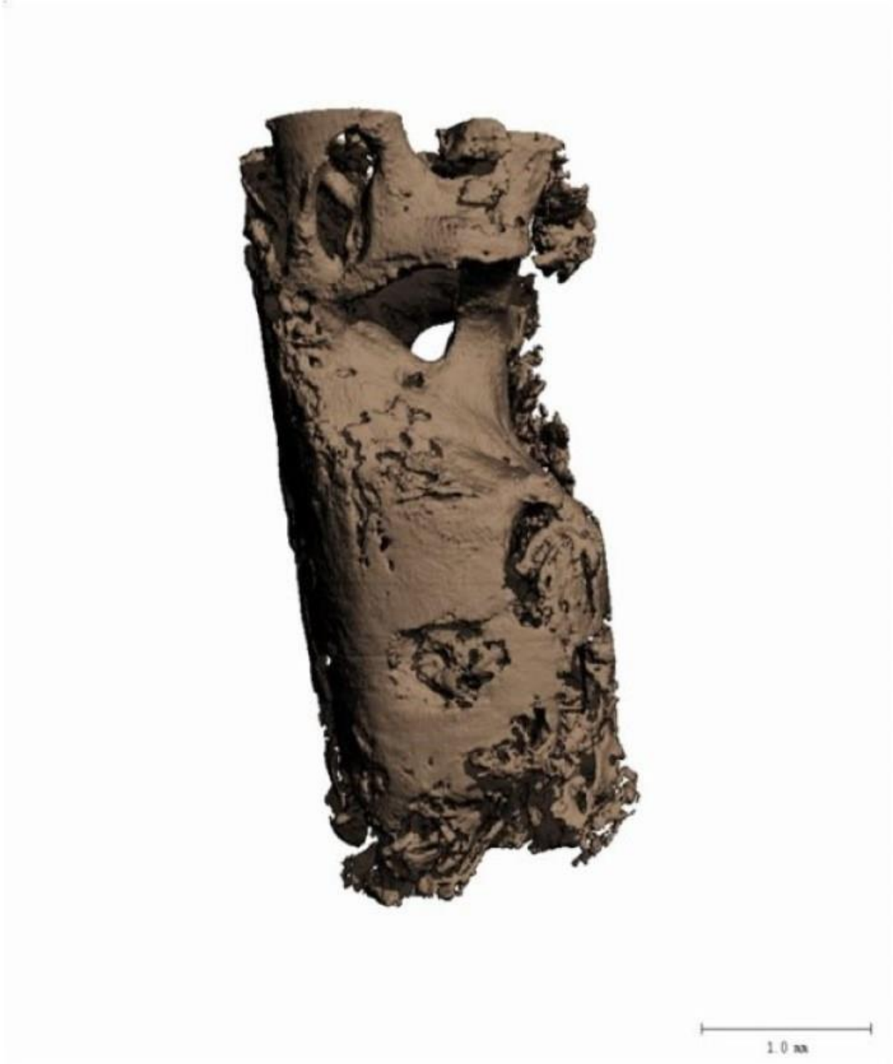
The core sample was evaluated with a micro CT scan to determine the morphology and physical characteristics of the bone generated 8 weeks after grafting with Socket Graft™.
